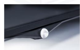
**4.** Connect **IR emitter** on the SoloCandy to the device's **infrared receiver.**
